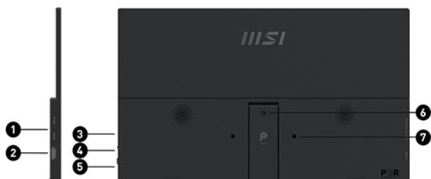
1. 2x Type-C (DP 1.2a signal with Alt mode & 15W Power Delivery / Power Input)
